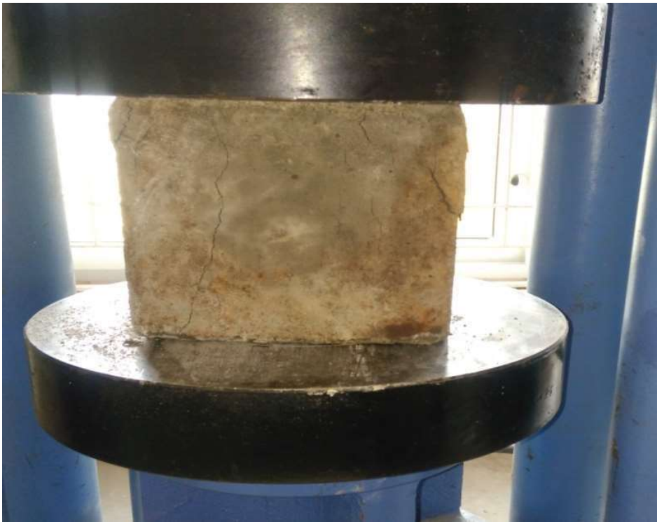
FIG 5.4 COMPRESSIVE STRENGTH TEST
