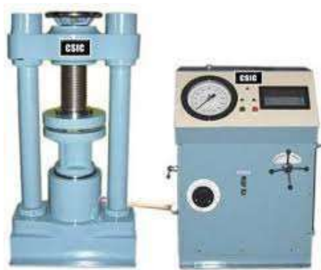
FIG 3.2 COMPRESSIVE TESTING MACHINE
