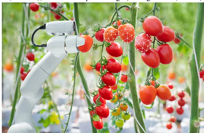
Figure 11: Automated harvesters use a combination of machine vision with a grasping tool to pick fruit and vegetables with precision. For some crops, this is relatively straightforward; for example, a robot harvesting wheat only needs to recognise the shape of rows planted in a field, which can be done by emitting lasers at the crop and measuring the reflection. Sources: Agro Robots | Which Robots Actually Work on Farms? | FoodUnfolded
