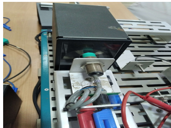
Figure 7: Magnetic sensor (Proximity sensor) aligned in front of the rotary target coupled with motor.
