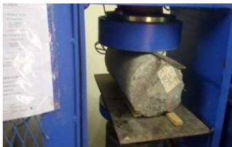
Fig. view of testing cylinder
