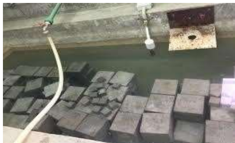
Fig. view of curing
