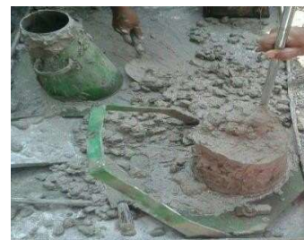
Fig. Testing of slump cone
