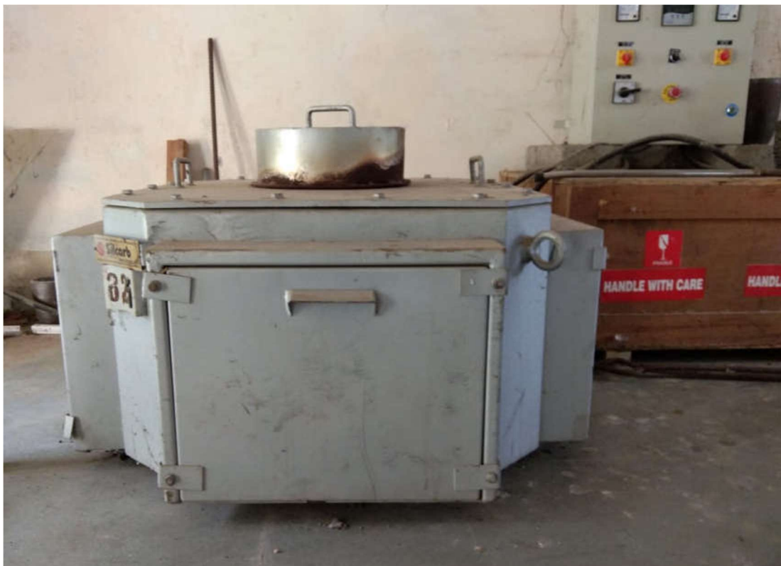
Fig.1 Electric resistance furnace with controll unit.
