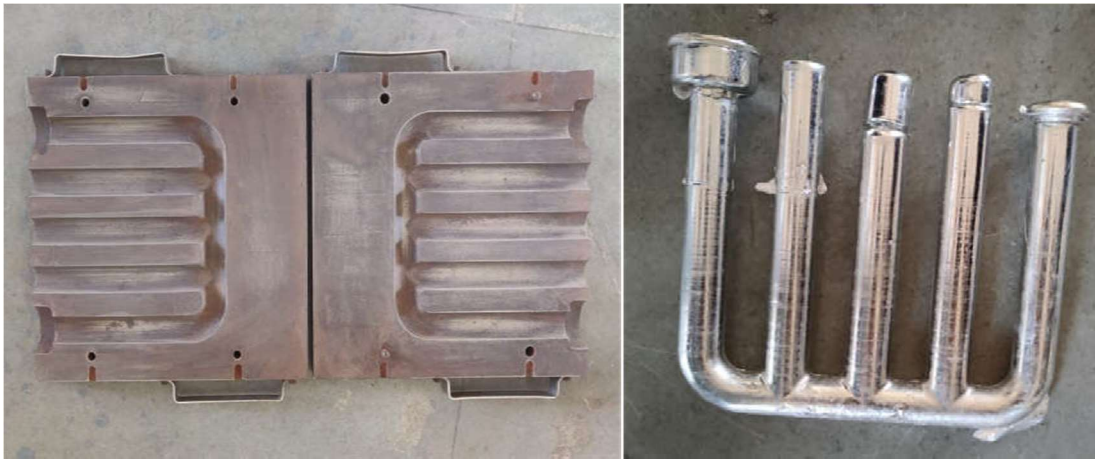
Fig.2 (a) Metallic Die (b) Casting after solidification
