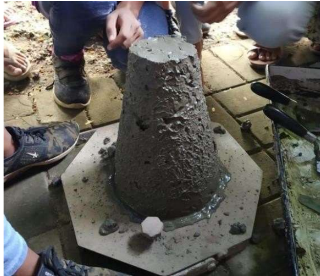
Figure: 2 Experiment work of slump test for checking slump value
