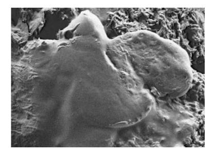
Ball-pen paste on laser printed document in the SUPRA<sup>TM</sup> 55. HV mode, 1 kV. No toner particle visible on the ball-pen paste is the proof of no falsification.
